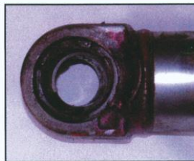
SEIZED PIN BUSHINGS INADEQUATE LUBRICATION
