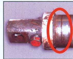
ABNORMAL WEAR IMPROPER USE OF CYLINDER OR UNAUTHORIZED ATTACHMENTS
