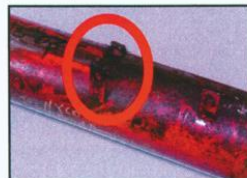
External welding on the cylinder customer modification.
