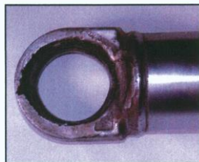
BROKEN PIN BUSHINGS INADEQUATE LUBRICATION
