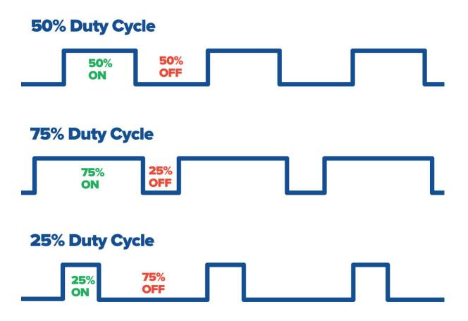
Suppose an automated side loader operator has a container close to an obstacle (such as a car or mailbox). In that case, the operator can use PWM technology in the joystick controls to slowly extend the arm, grab the container, dump it, and replace the container with much more finesse than if the arm went out at full speed. PWM can also reduce the cab shake that causes driver fatigue by allowing a much smoother lift arm function over running the lift arm at 100% speed.
