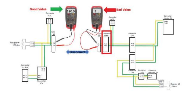
We disconnected connector ARM2 and tested resistance in both directions. We have good resistance in one direction and a bad value in the other. We will follow the direction of the incorrect resistance
