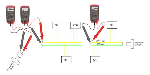
If an open circuit is found, this would be a good indication you have a broken wire or a poor connection at a connector.
