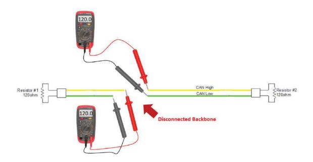
If we disconnect one or all of the ECUs on a single network, this should not change the known resistance of the backbone's  $60\Omega$ .
