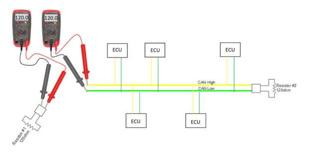
If you have two disconnects on the backbone, you will only have  $120\Omega$  resistance on wires connected to the resistor. If no resistor is found, your meter will display 1, indicating an open circuit.
