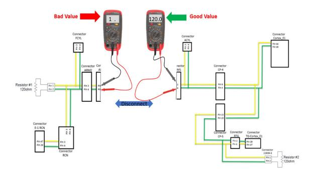
Now at the ARM1 connection, we find a good resistance on the right, and the side that had a good resistance now has a bad value. We know we have just passed the wiring problem. The problem is between the ARM2 and ARM1 connections. It could be a broken wire, rodents chewed into the harness, or maybe even a pin that is corroded or pushed out of the harness connector.
