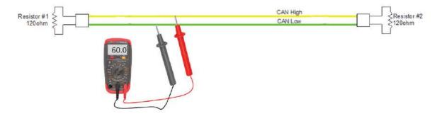
The meter shown above is for reference to the resistance in the network only. DO NOT PIERCE THE BACKBONE OF THE NETWORK WITH METER LEADS!
