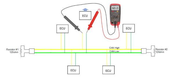
Another good place to test is at the terminating resistor connector. Disconnect the resistor and check the resistance. This will measure resistance from one end to the other. Don't forget to check the resistor as well.
