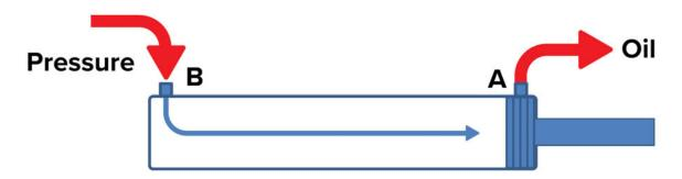
To properly diagnose for cylinder bypass, the cylinder needs to be checked in both directions for bypass by reversing the test procedure.
