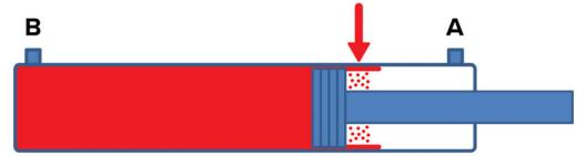
To prevent this from happening, we need to be sure that we are maintaining the hydraulic system by keeping leaks contained, and the oil clean by being careful when opening the system to fill or inspect, preventing side loading, maintaining proper system pressures, and by also adhering to the filter and oil change intervals recommended in the Heil Service Manual.
