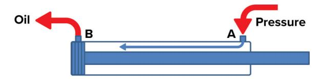
If more than 8oz of hydraulic oil bypasses the piston, the cylinder will need to be replaced or rebuilt to restore its full functionality. If you have cylinder bypass questions, please feel free to email or call the Heil Technical Service Team with the following contact information.
