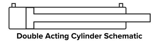
When a cylinder is "bypassing," the hydraulic oil "bypasses" the seals on the piston to the other side of the cylinder when pressurized. This can cause the hydraulic function to be slow and can cause erratic hydraulic functionality. 3 to 8oz per minute is considered an acceptable amount of oil bypass. When checking for bypass, keep in mind that If the oil bypass is above 8oz per minute, the cylinder should be rebuilt or replaced.
